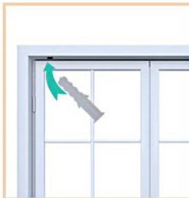
03. Plug the expansion screw into holes
